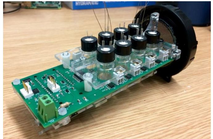
Fig. 5. Internal PCB of aroma generator.
