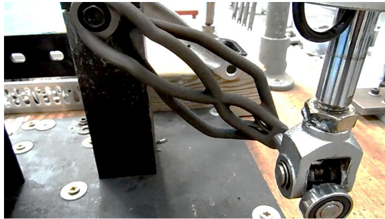
Figure 8. Fatigue Test Configuration.
