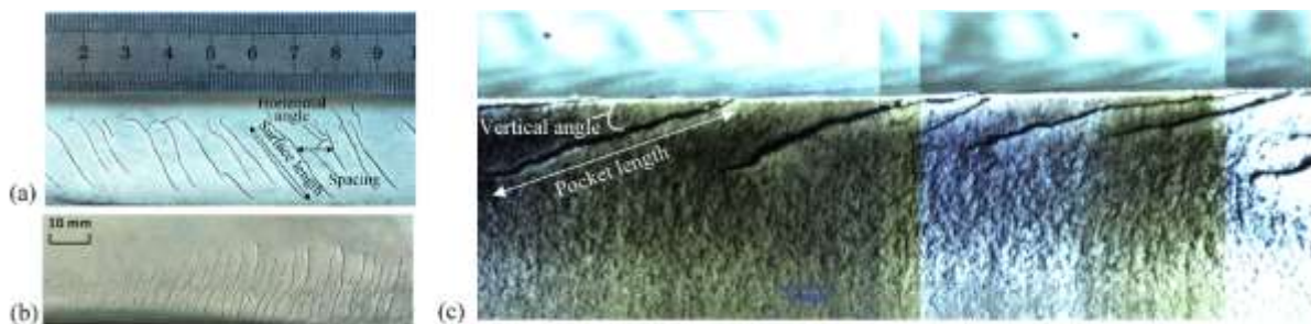
Figure 1 (a) Magnetic particle inspection (MPI) image showing RCF crack clusters on a rail sample taken from service; (b) MPI image of RCF cracks showing non-uniformly distributed cracks along the rail running direction; (c) a cross section of a crack cluster showing the cracks propagating into the rail.
