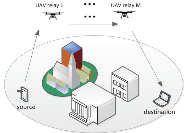
FIGURE 1. A multi-hop UAV relaying communication system.
