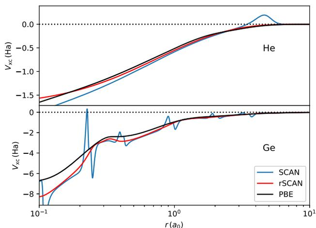
**FIG. 4.** Multiplicative part of the SCAN and rSCAN exchange-correlation potentials computed using the PBE self-consistent electronic and kinetic energy densities of isolated He (top) and Ge (bottom) atoms. The PBE result is also shown for reference.
