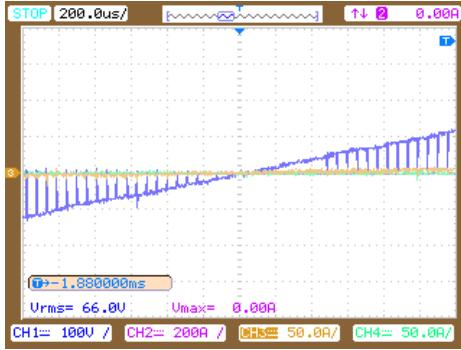
Fig. 5.  $v_r$  around voltage zero-crossing range.
