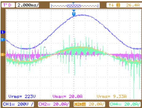
Fig. 6. Voltage regulation in experiment (CH1:  $v_{ou}$ , CH2:  $i_B$ , CH3:  $i_{ou}$ , CH4:  $i_T$ ).
