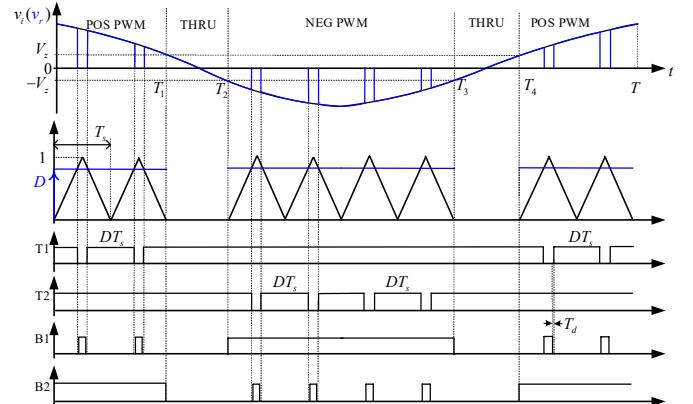
Fig. 2. PWM control of ac-ac buck converter.
