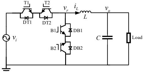
Fig. 1. Single-phase PWM ac-ac buck converter.
