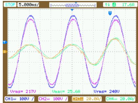
Fig. 4. Voltage regulation in experiment with a step change in load (CH1:  $v_{in}$ , CH2:  $i_{in}$ , CH3:  $v_{ou}$ , CH4:  $i_{ou}$ ).
