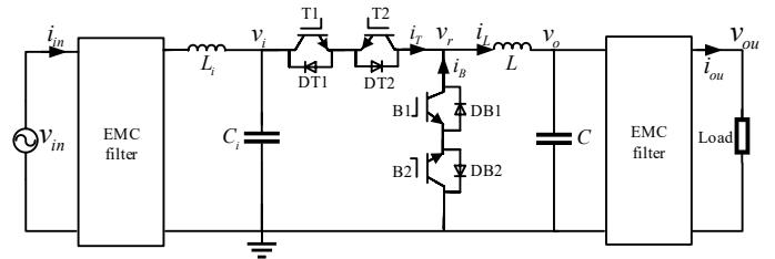
Fig. 3. Circuit diagram of the system based on the PWM ac-ac buck converter.
