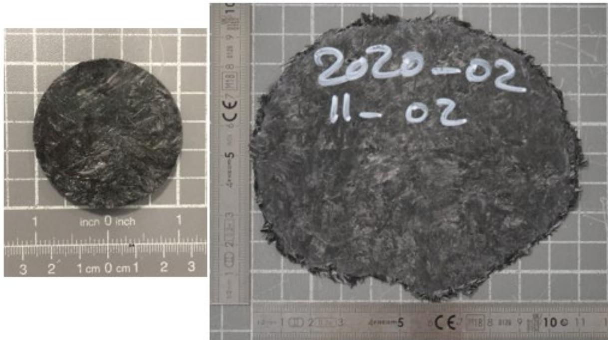
Fig. 2: An example squeeze flow testing sample tested at 80°C and 2mm/s closing speed.
