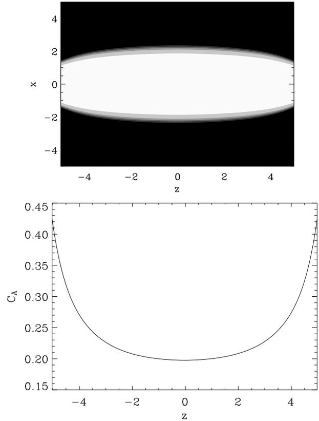
**Fig. 2.** *Top*: contour plot of the density profile that is added on top of the magnetic field profile shown in the *bottom* panel of Fig. 1. A generalised symmetric Epstein profile with steepness parameter  $p = 10$  is used, along with a varying semi-width parameter  $a(z)$  chosen to follow a particular field line. *Bottom*: the Alfvén speed profile along the loop axis.
