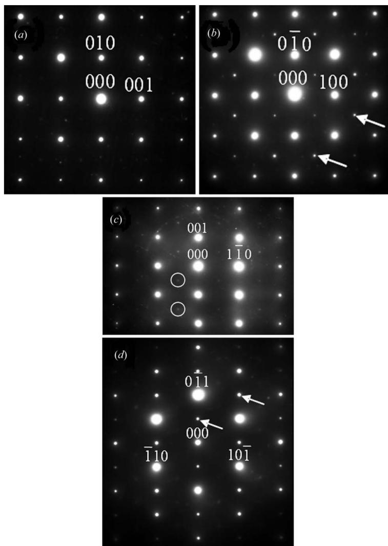
**Figure 12** Diffraction patterns obtained from an NBT sample at 713 K. These are indexed with zone axes (a) [100], (b) [001], (c) [110] and (d) [111]. Superlattice reflections arising from in-phase tilting are arrowed. Weak superlattice reflections possibly arising from antiphase tilting are ringed.
