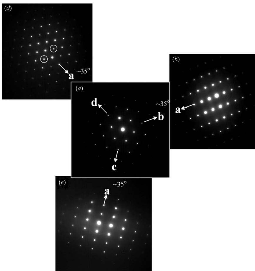
**Figure 8** Results of tilt experiment for  $BiFeO_3$ . (a) The central  $\langle 111 \rangle$  ZADP, (b) and (c)  $\langle 110 \rangle$  ZADPs without superstructure reflections, (d)  $\langle 110 \rangle$  ZADP with superstructure reflections (ringed). The labelled arrows indicate the orientational relationship between these diffraction patterns.
