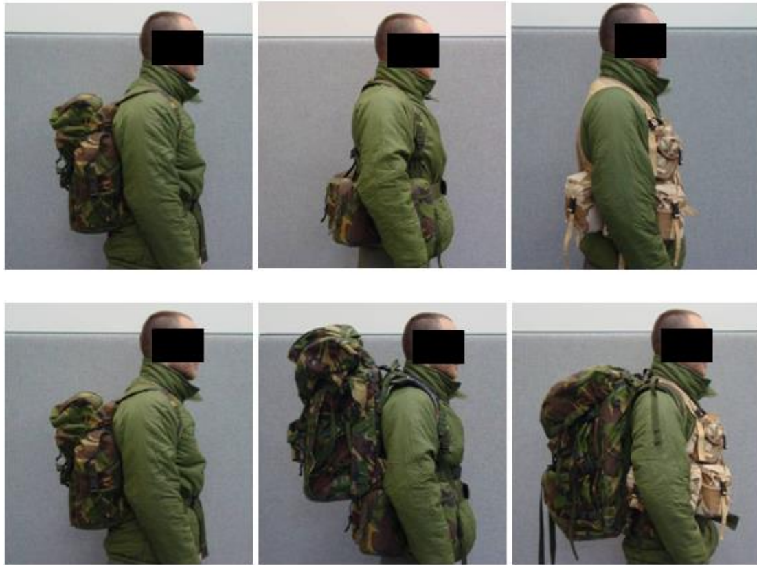
Figure 1: Backpack, Standard and AirMesh LCS (left to right respectively, top and bottom). Top three images show LCS setup when 8 or 16 kg were carried, bottom three images when 24 or 32 kg were carried.
