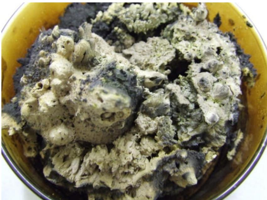
*Figure 4.1. Result of drying the viscous sol in a standard 115mm diameter dish. As the solvents in the sol evaporated and expanded they were unable to break the surface tension, resulting in an expansion of the sol.*
