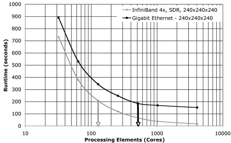
**Figure 4:** Chimaera Runtime using InfiniBand (4x, SDR) and Gigabit Ethernet Interconnects.
