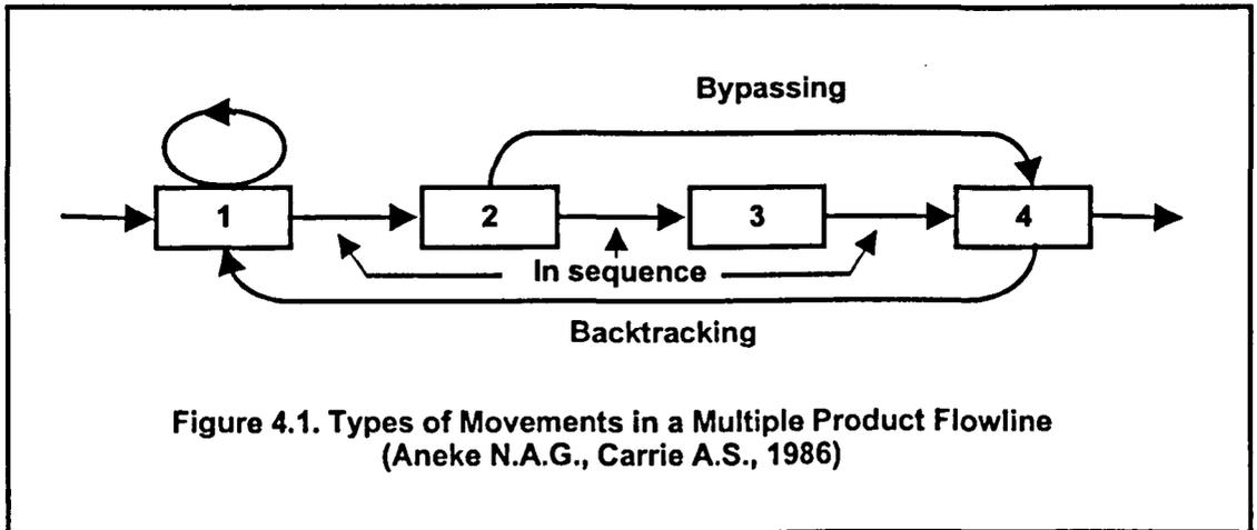
Figure 4.1. Types of Movements in a Multiple Product Flowline
