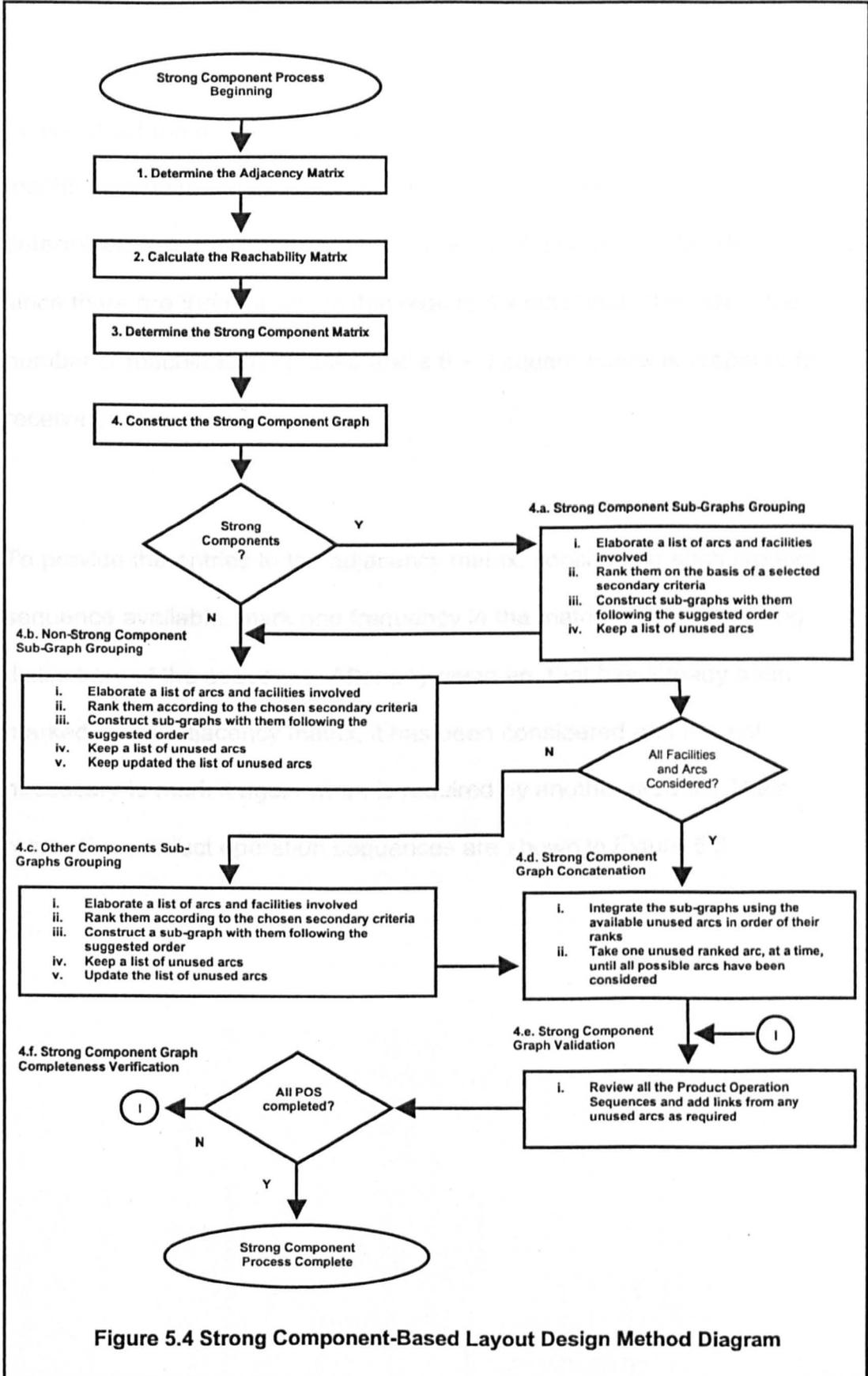
Figure 5.4 Strong Component-Based Layout Design Method Diagram
