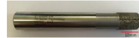
Fig. 1. 10mm diameter of nickel layer electroplated cutting tool with average of 420 \mu m diamond grit.
