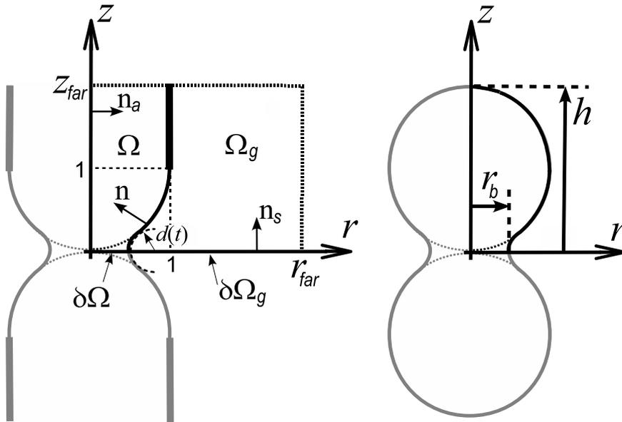
FIGURE 2. A definition sketch for the coalescence of two identical ‘pinned hemispheres’ grown from syringes (left) and a sketch of coalescing ‘free spheres’ (right) showing the bridge radius  $r_b$  and apex height  $h$ . In the results section, the bridge radius will simply be denoted as  $r$ .
