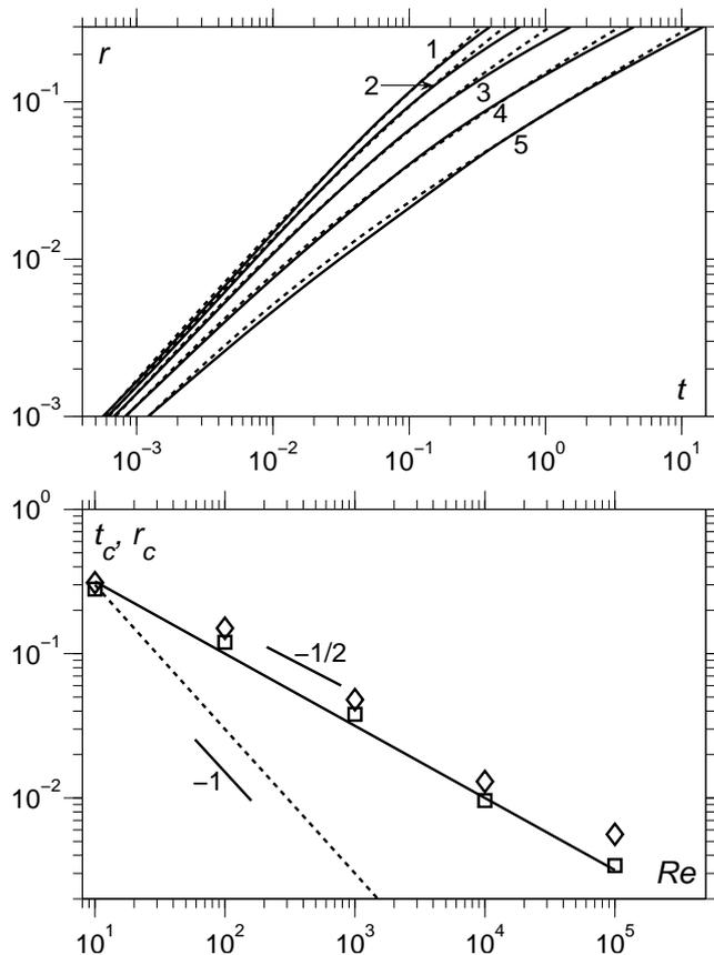
FIGURE 14. Effect of the  $Re$ , with  $\bar{\mu} = 4.6 \times 10^{-5} Re^{1/2}$  for the case of a varying viscosity. Curve 1:  $Re = 10$ , curve 2:  $Re = 10^2$ , curve 3:  $Re = 10^3$ , curve 4:  $Re = 10^4$  and curve 5:  $Re = 10^5$ . Dashed lines are equation (7.2) with constants that are plotted in the lower figure: diamonds are  $t_c$  and squares are  $r_c$ .
