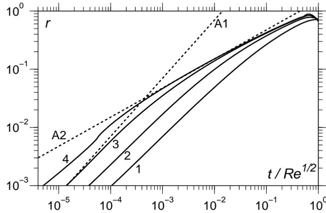
FIGURE 7. Curves from Figure 5 plotted against the time scaled using  $T_i$ , i.e.  $r$  against  $t_i = t/Re^{1/2}$ , characteristic of the inertia-dominated regime as opposed to  $T_v$  in Figure 5. Curve 1:  $Re = 10^1$ , 2:  $Re = 10^2$ , 3:  $Re = 10^3$  and 4:  $Re = 10^4$ . The dashed line A1 is for (2.5), i.e. a linear curve ( $r = 70t_i$ ) and A2 is for (2.4), i.e. the scaling  $r = 1.5t_i^{1/2} = 1.5t_i^{1/2}/Re^{1/4}$
