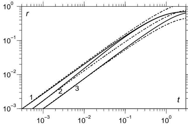
FIGURE 13. An illustration of the influence of the gas viscosity on the coalescence of drops (with  $Re = 0$ ). Curve 1:  $\bar{\mu} = 0$ , 2:  $\bar{\mu} = 10^{-4}$  and 3:  $\bar{\mu} = 1$ . The top dashed line correspond to (2.1) whilst the middle and lower ones are the same expression with a *fitted* prefactor of 0.6 and 0.35, respectively.
