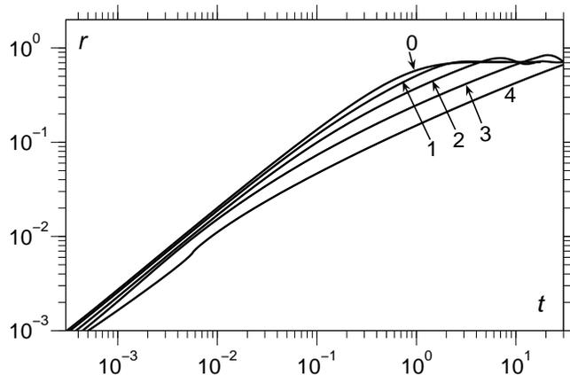
FIGURE 5. Bridge radius as a function of time for a variety of different Reynolds numbers. Curve 0 is for  $Re = 0$  (curves for  $Re \leq 1$  are graphically indistinguishable from it), 1:  $Re = 10^1$ , 2:  $Re = 10^2$ , 3:  $Re = 10^3$  and 4:  $Re = 10^4$ .
