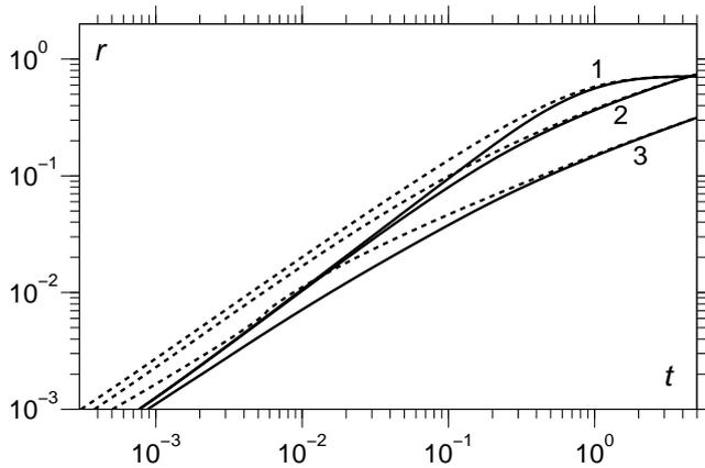
FIGURE 12. The effect of the Reynolds number on the time-dependence of the radius of the bridge connecting the coalescing drops calculated for a fixed viscosity ratio  $\bar{\mu} = 10^{-2}$  (solid lines) compared to the  $\bar{\mu} = 0$  case (dashed lines) with curve 1:  $Re = 0$ , curve 2:  $Re = 10^2$  and curve 3:  $Re = 10^4$ .
