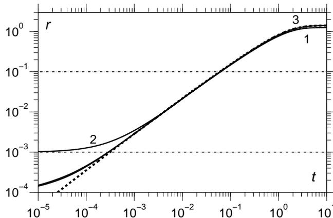
FIGURE 3. Bridge radius as a function of time for the case  $Re = 0$  compared to Hopper's solution (2.1), the dashed line. Curve 1 is for three-dimensional free spheres with  $r_{min} = 10^{-4}$ , curve 2 the same except that  $r_{min} = 10^{-3}$  and curve 3 is for two-dimensional free cylinders ( $r_{min} = 10^{-4}$ ).
