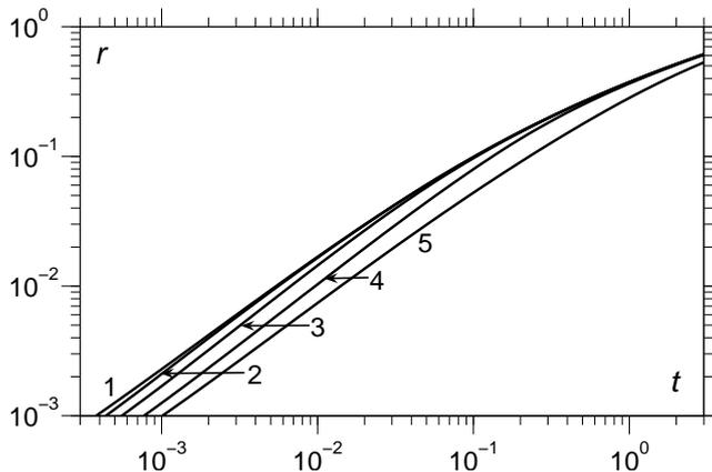
FIGURE 11. Influence of gas viscosity on the time-dependence of the radius of the bridge connecting the coalescing drops calculated for fixed  $Re = 10^2$  with curve 1:  $\bar{\mu} = 0$ , 2:  $\bar{\mu} = 10^{-6}$ , 3:  $\bar{\mu} = 10^{-4}$ , 4:  $\bar{\mu} = 10^{-2}$  and 5:  $\bar{\mu} = 1$ .
