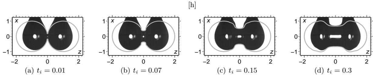
FIGURE 1. Comparison of our coalescence computations with free spheres in the inertial regime, against experiments in Paulsen *et al.* (2012) conducted using 1 mm radii pendant drops of silicone oil with  $Re = 1.9 \times 10^4$ . The dimensionless time  $t_i$  is based on the inertial scale. As can be seen, the neck region is accurately described far beyond the initial stages of the process even though the global geometry is different.
