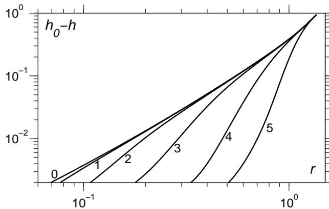
FIGURE 8. Distance  $h_0 - h$  that the apex has moved plotted against bridge radius  $r$  for different Reynolds numbers. Curve 0:  $Re = 0$ , curve 1:  $Re = 10^{-3}$ , 2:  $Re = 10^{-2}$ , 3:  $Re = 10^{-1}$ , 4:  $Re = 1$ , curve 4:  $Re = 10$  and curve 5:  $Re = 10^2$ .
