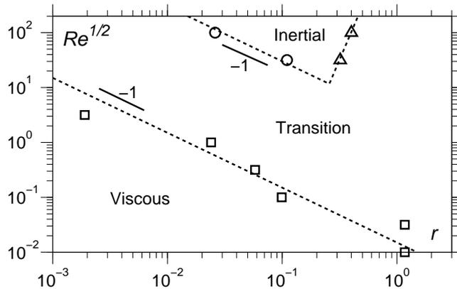
FIGURE 16. Phase diagram showing the regions in which the bridge radius  $r$  is in the viscous regime described by (2.1) or in the inertial regime described by (2.4) with  $C_i = 1.5$ . Dashed lines are rough fits to the data with the lower dashed line given by  $Re^{1/2} = 1.5 \times 10^{-2} r^{-1}$ , upper dashed line (with gradient  $-1$ ) is  $Re^{1/2} = 3r^{-1}$  and the third dashed line, going through the triangles, is simply to guide the eye.
