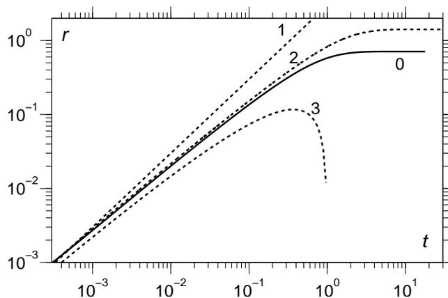
FIGURE 6. Comparison of the full numerical solution for  $Re = 0$  (and hence all  $Re \leq 1$ ) curve 0 with scalings and the exact solution for free cylinders. Curve 1: linear plot (2.5) of  $r = 3t$ ; curve 2: Hopper's solution for free cylinders (2.1); curve 3: formula (2.3) for a passive gas, i.e.  $r = -(1/\pi)t \ln t$ . It is clear that Hopper's solution best approximates the full numerical solution.
