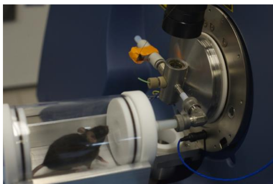
Fig. S1. Experimental set-up. The vapors emitted by a mouse after being injected with ketamine were constantly sampled using 2 L/min of medicinal air through the mouse chamber. Gas-phase analytes (i.e., ketamine and its metabolites) entered the SESI source attached to the curtain plate of the mass spectrometer. Full mass spectra were recorded in the range m/z 100-400, allowing to capture pharmacokinetic profiles in real-time with a time resolution of 5 s.
