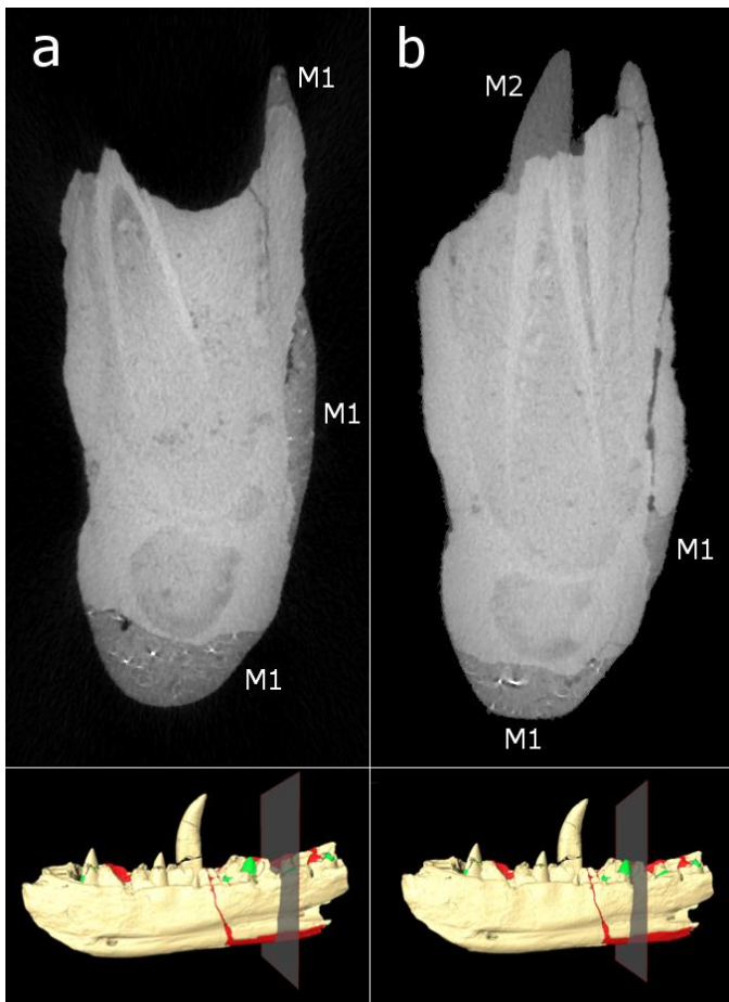
Fig. 3. Identification of Plaster Materials from XCT Data. a ) Identification of Material 1 (M1). b ) Identification of Material 2 (M2) alongside M1. Both materials can be easily differentiated from each other. Insets representative of slice location.
