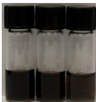
Figure 3. Photograph of P3 -SWNT prepared with a polymer:nanotube mass ratio of (left to right) 2.5:1, 5:1, or 10:1 in a 50/50 mixture of THF:DMF.
