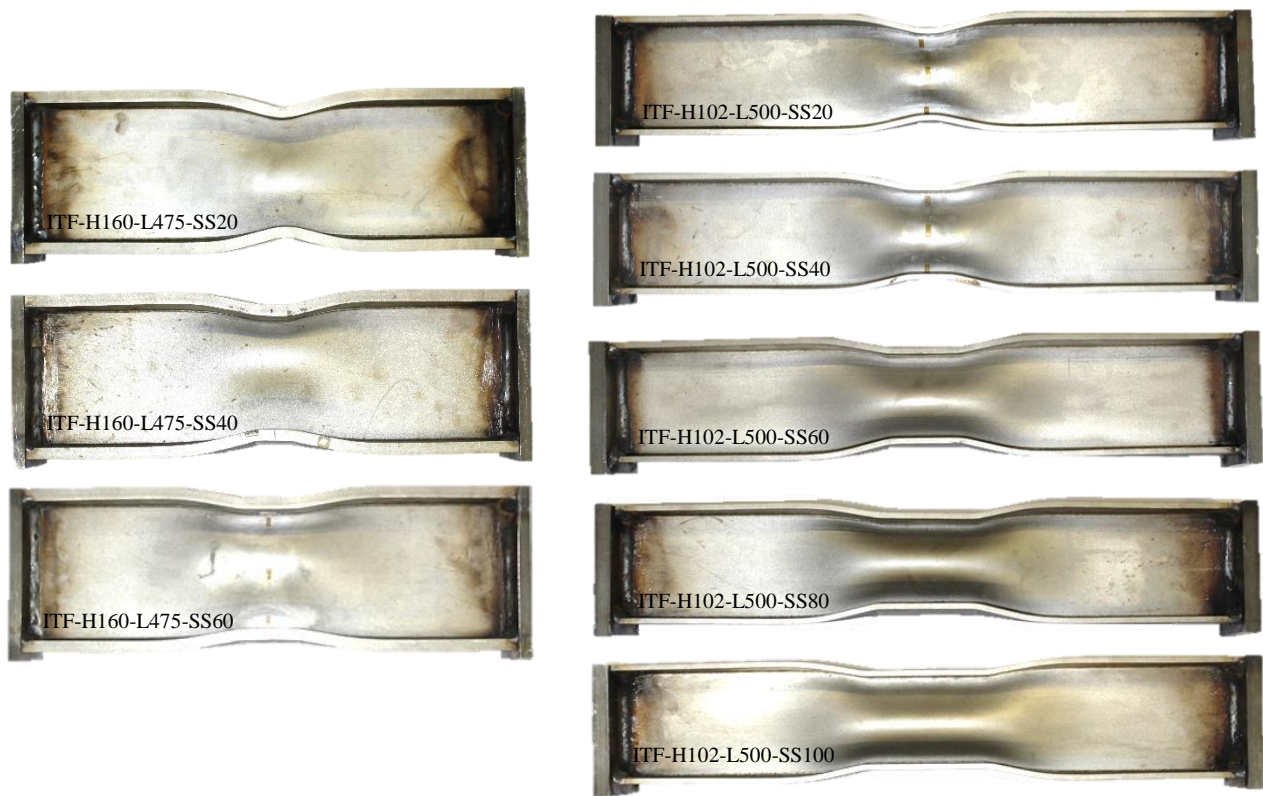
Fig. 16. Failure modes of internal two-flange (ITF) loading test specimens.
