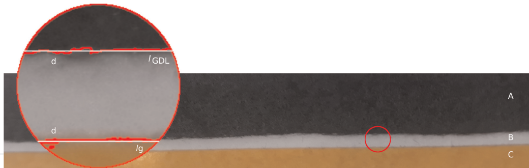
Figure 2. GDL (A), gap (B), gasket (C), edges (d), straight line fitted to each edge ( l_g and l_{GDL} ).
