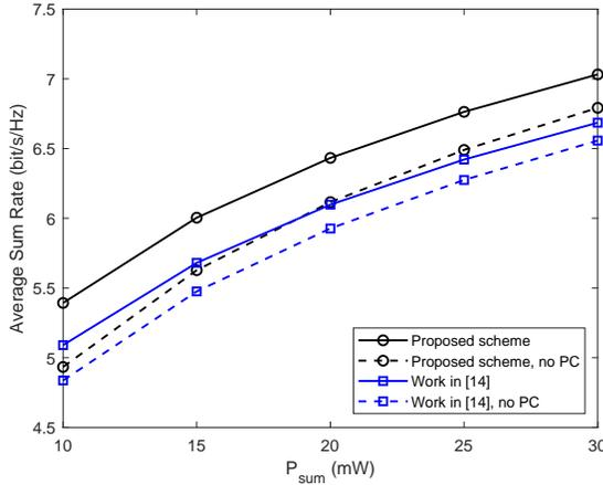
Fig. 3. Average sum rate comparison of the proposed scheme and the scheme in [14].
