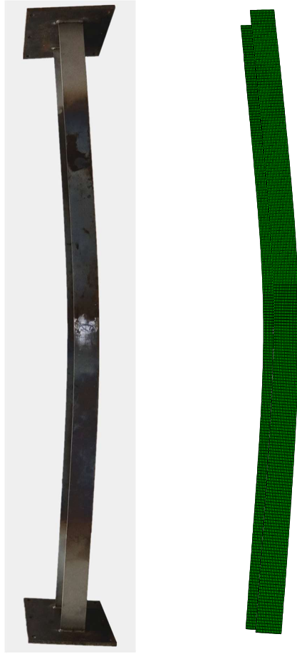
Figure 2: Experimental and numerical failure modes for specimen BC-Z10-0.4 [15]
