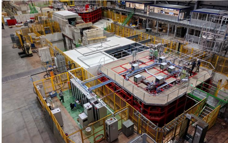
Figure 3.12: The EHN1 building extension at CERN's Preveessin site - home to the two ProtoDUNEs. ProtoDUNE-SP can be seen in the foreground, while ProtoDUNE-DP is in the background. Located between the two detectors, surrounded by the large concrete blocks, is the end of the H4 beamline pointing towards ProtoDUNE-SP.
