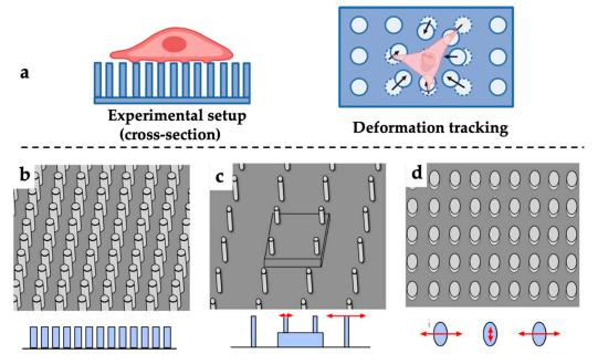
**Figure 2.** Schematics of EMP. (**a**) Methodology for cellular force sensing with EMP; (**b**) Tightly arranged short micro-pillars; (**c**) Loosely arranged micro-pillar matrix with varying heights; (**d**) Anisotropic pillar designs arrays.
