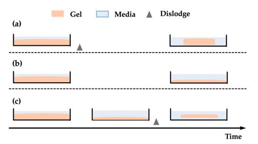
**Figure 3.** Schematics showing the variation of contraction assays based on dislodge time. (**a**) Immediate dislodge; (**b**) No dislodge; (**c**) Dislodge after a period of time.
