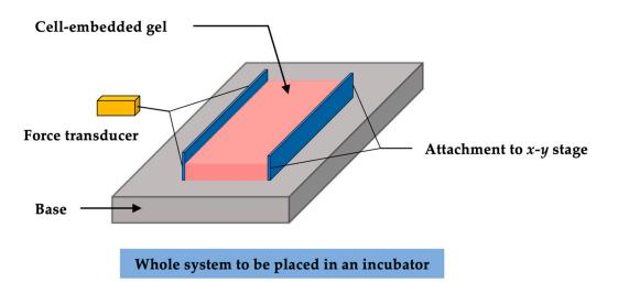
Figure 5. Schematic diagram of a typical CFM system.
