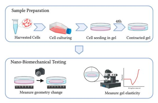
Figure 4. Schematic shows the methodology of the new nano-biomechanical technique for cellular force measurement.
