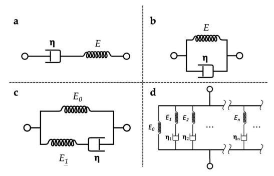
**Figure 6.** Schematics of typical constitutive models for viscoelastic materials. (a) Maxwell model; (b) Kelvin-Voigt model; (c) Standard linear solid (SLS) model; (d) Maxwell-Wiechet model. *E* and  $\eta$  are the elastic modulus of the elastic spring element and the viscosity of the damper element respectively.
