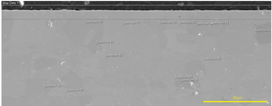
Figure 5.56 Fe-3Al-5Mn, Humidifier 0°C, 20-30sec second run. SEM image 10µm scale view, with spectra analysis
