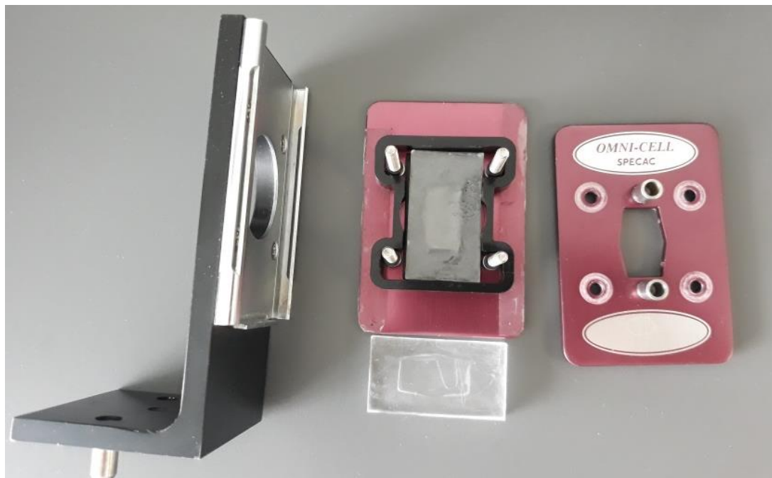
Figure 3.8. Transmission cell from Specac and NaCl windows.
