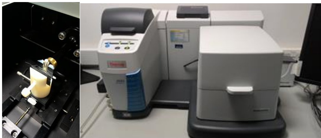
Figure 4.9. Picture of the DXR Smart Raman Spectrometer: sample holder (a) and outside (b)
