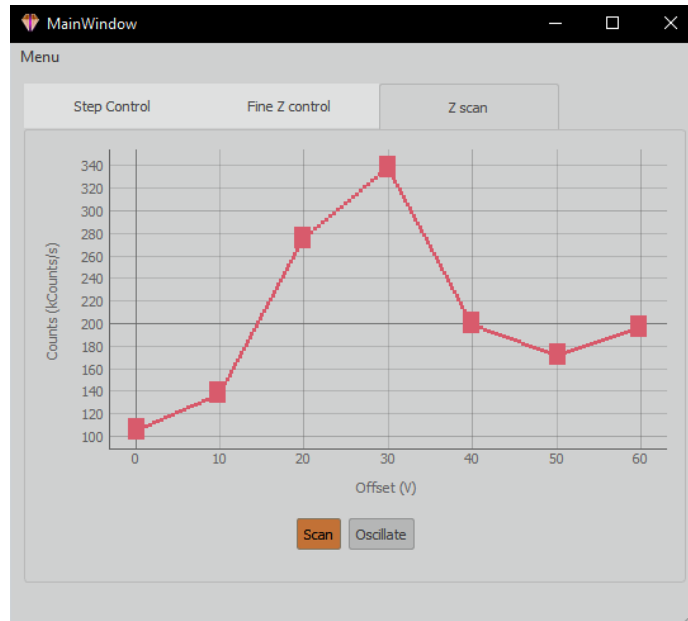
Figure 3.12: The Qudi version of the Attocube positioner control GUI. Scanning through a surface or a fluorescing point source such as a nanodiamond gives a peak which can be fitted. Given the limited scan range, fitting can be ambiguous so the focus needs to be updated frequently enough to track the focus until any movement slows after changes.
