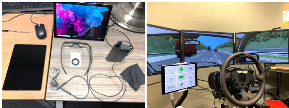
FIGURE 35 APPARATUS USED IN IUS2. PICTURED IS THE IPAD PRO, TOBII PRO 2, SURFACE PRO, CALIBRATION CARD, SCREEN CLEANING CLOTH AND BLUETOOTH HEADPHONES USED TO CONTROL INFORMATION DISPLAY PLAYBACK
