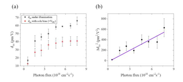
**Figure 4.** Analysis of underlying mechanisms behind light-induced  $d_{zz}$  enhancement. (a) Comparison of  $d_{zz}$  measured only under illumination and application of a  $V_{dc}$  (=  $V_{oc}$  of the corresponding photon flux), and (b) their differences of  $d_{zz}$  squared ( $\Delta d_{zz}^2$ ), showing a linear relationship with the increased photon flux.
