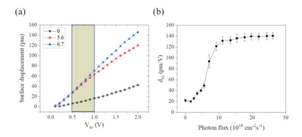
**Figure 2.** Quantitative analysis of piezoelectricity under illumination. (a) Surface displacement versus  $V_{ac}$  curves, wherein the inset shows the photon flux in the unit of  $10^{18}$  cm<sup>-2</sup>s<sup>-1</sup>. Slopes of these curves measured in yellow region indicate the effective piezoelectric constants,  $d_{zz}$ . (b) Evolution of the 15 representative  $d_{zz}$  values with increasing the photon flux.
