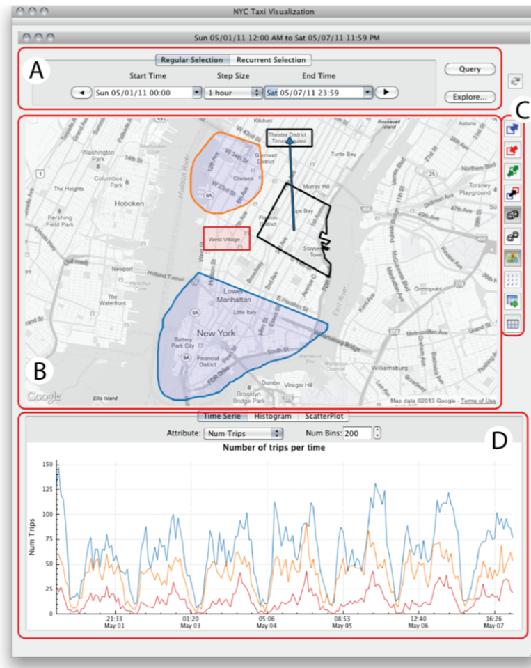
Figure 1.5 The TaxiVIS project, demonstrating the various user interface components. (A) Time selection widget, (B) Map, (C) Tool bar, and (D) Data summary (Ferreira et al., 2013, p. 2152)
