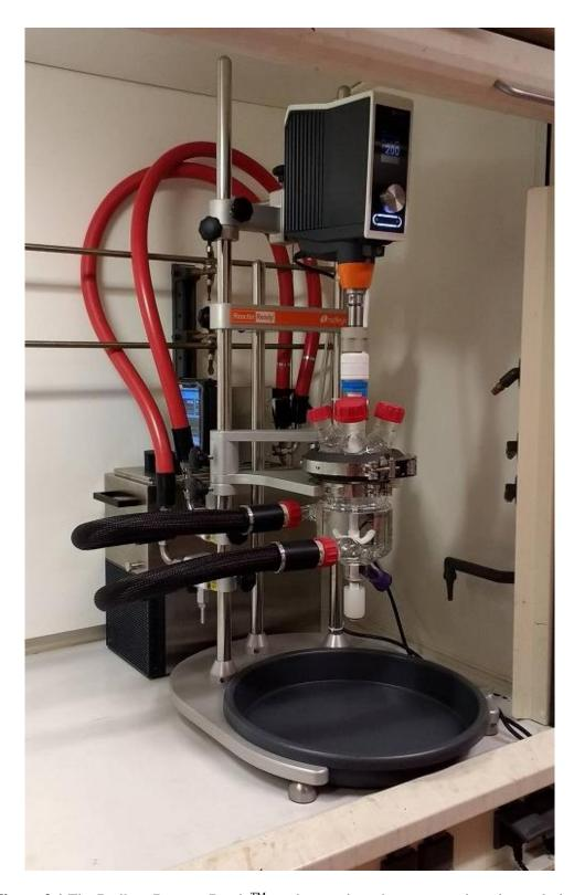
**Figure 2.1** The Radleys Reactor-Ready<sup>TM</sup> used to produce the aqueous zirconium solutions studied in this project. Not pictured is the water-cooled condenser. The oil heating and circulating equipment is positioned sideways behind the reactor vessel stand, connected to the vessel via two pairs of insulated hoses. The top of the temperature probe is just visible behind the upper rotating parts of the overhead stirrer.
