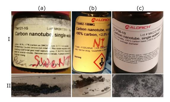
Figure 2.1: The different types of SWCNTs utilised in this research, as sourced from the supplier (Sigma Aldrich). The (a) SWeNT, (b) NI, and (c) CHASM SWCNTs were supplied in (I) sealed glass containers - with basic compositional details noted on the labels - as (II) powder or flakes.
