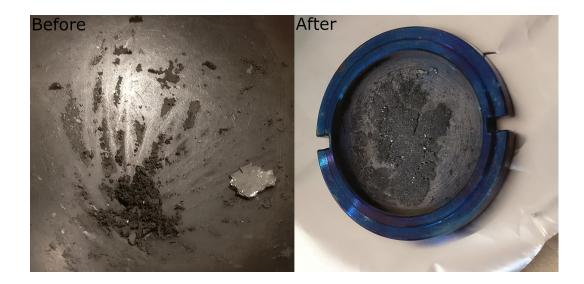
Figure 3.24: Images of the as-supplied bulk  $Sb_2Te_3$  prior to, and immediately after, heating under nitrogen atmosphere and cooling to room temperature, using the static stage XRD configuration. The as-supplied bulk sample was finely ground prior to XRD. Visual inspection of the post-experiment sample showed the heat cycling to have caused shrinkage to centre of holder, and a loss of mass. This resulted in significant portions of the steel alloy holder becoming exposed.
