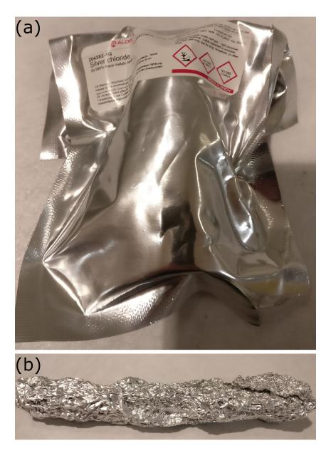
Figure 2.5: Packaging and experimental considerations for light sensitive materials. (a) Silver chloride is supplied in opaque, reflective packaging to minimise risk of light exposure. (b) When not in a red-lamp environment, the sample must be wholly encased in light-blocking material. In this case, the entire double ampoule is encased in foil for the sublimation growth stage, and during any portion of the preparation that is not conducted in a dark room.
