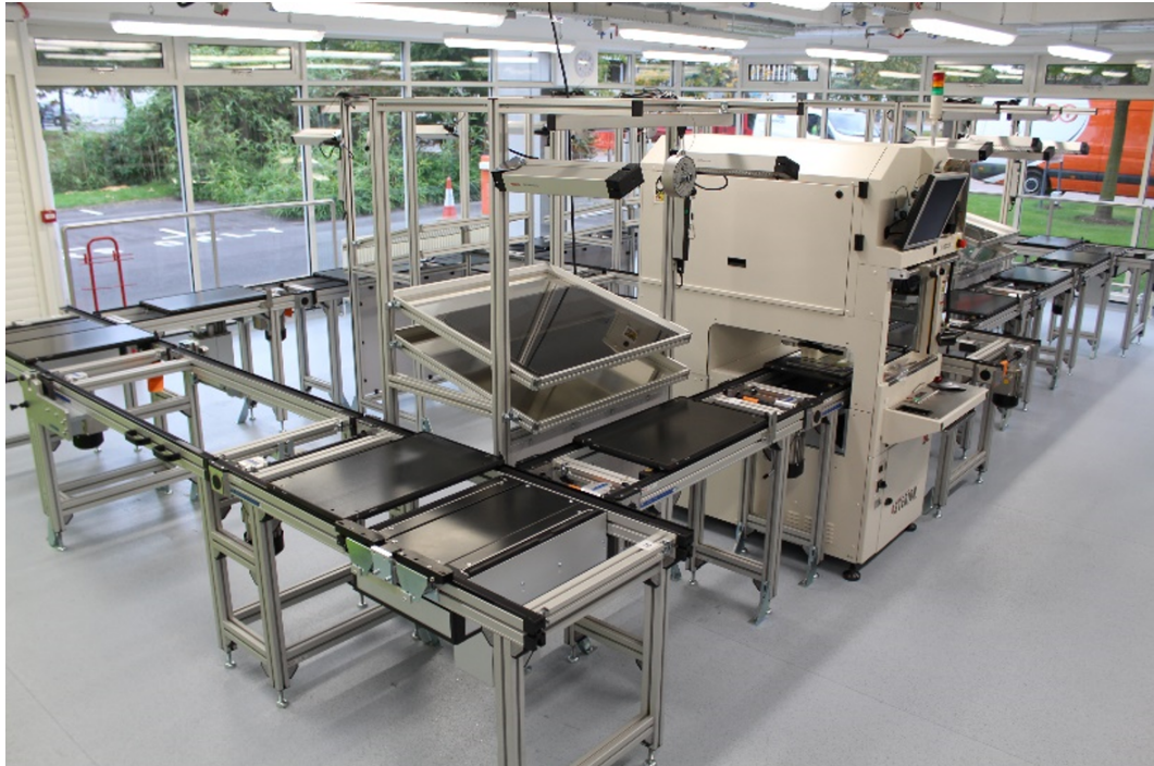
Figure 4.1: Pilot line for battery module assembly in WMG.
