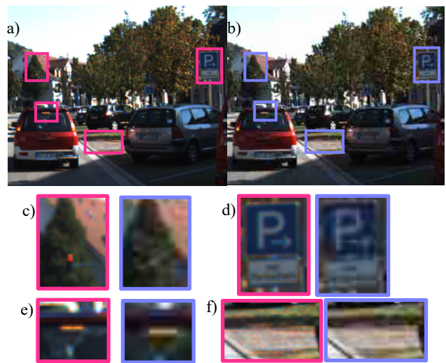
Figure 3. A selected area from one frame of KITTI MoSeg dataset, (a) uncompressed, (b) maximum compression; the rectangles in a) and b) highlight the details which are zoomed: c) traffic light (not visible on the right), d) brake lights (intensity degraded on the right), e) P sign characters (distorted on the right), f) parking slot (blocky artifacts on the right). In c), d), e) and f) the details from the frame uncompressed and with maximum compression are on the left and right sides respectively.
