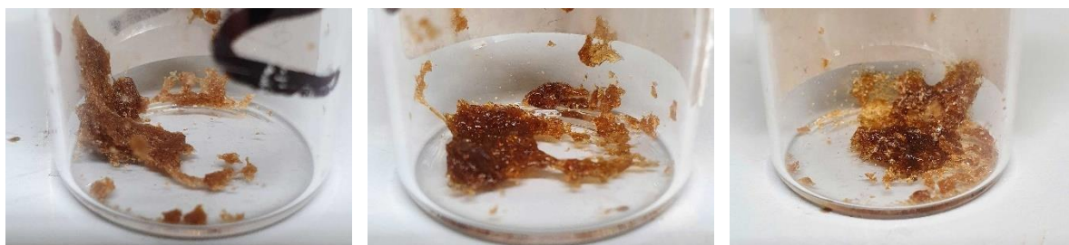
Figure 3.2.5.9: Isolated and dried PVAc, formed after acetylation of PVOH. DVA (100/1/1) (left), No comonomer (100/1/0) (centre), and BDDVE (100/1/1) (right).
