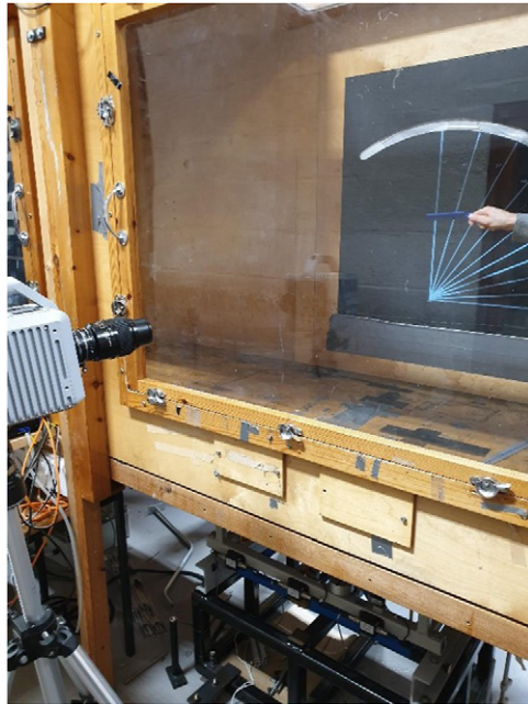
Figure 1. Image of the experimental wind tunnel set-up and high-speed camera. A piece of acrylic has been used as a reference. Note that the object is not clamped in place and that it is instead moved by hand to imitate a typical flapping-twisting motion.
