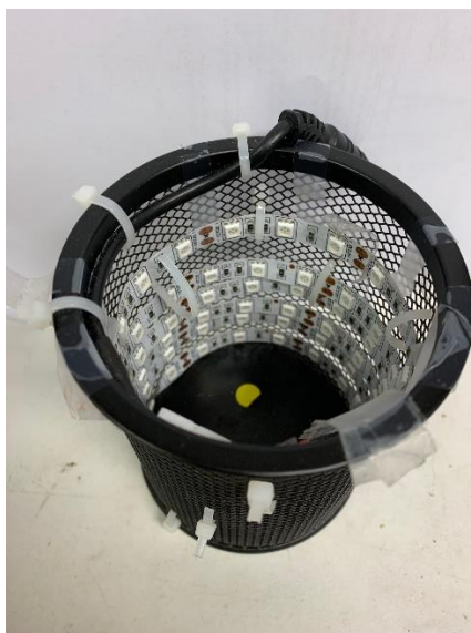
Figure 2.10 LED reactor used for photoiniferter reactions.
