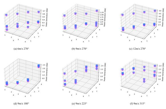
Fig. 4. The qualitative comparison between the predicted result and the ground truth. The magenta circle indicates the ground truth generated by the FLORIS, the dodger blue triangle denotes the result predicted by the WiT, and horizontal and vertical coordinates represent the spatial position of the corresponding turbine.
