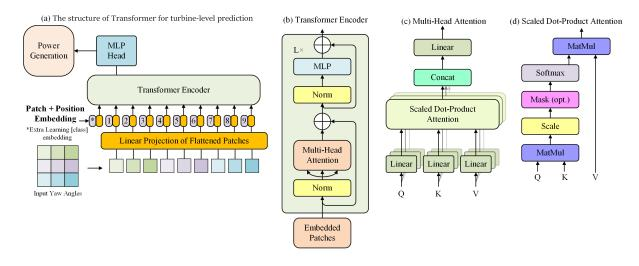
Fig. 2. The illustration of the Wind Transformer (WiT). (a) The structure of Transformer for wind farm prediction. (b) Transformer Encoder. (c) Multi-Head Attention. (d) Scaled Dot-Product Attention.
