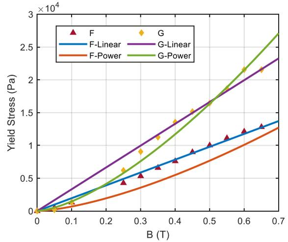
Fig. 4. Linear and power laws in comparison with the experimental yield stresses for: left) samples D and E, right) samples F and G.
