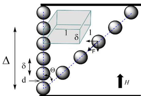
Fig. 2. Pre-yield chains deformation under an external magnetic field and a shear stress.
