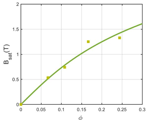
Fig. 6. Variation of the model parameters with the volume fraction of CIP.
