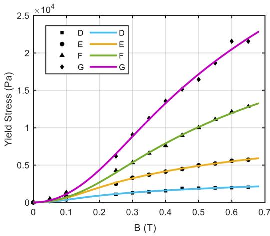
Fig. 5. Yield stresses of the MRF samples; comparison of the model results with the experimental data.
