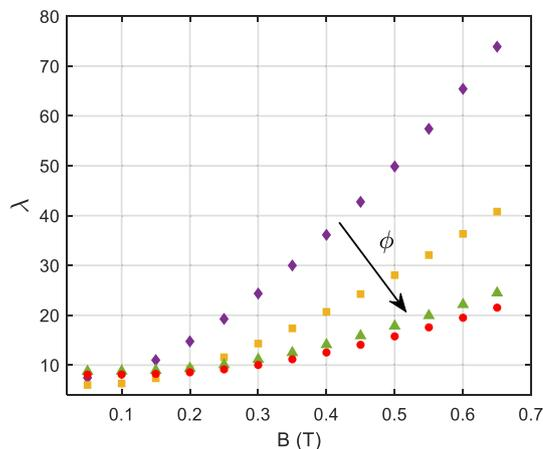
Fig. 8. The rate parameter of exponential PDF calculated for the MRF samples.
