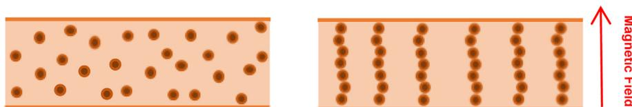
Fig. 1. Schematic of an MRF in off-state (left), and on-state (right).
