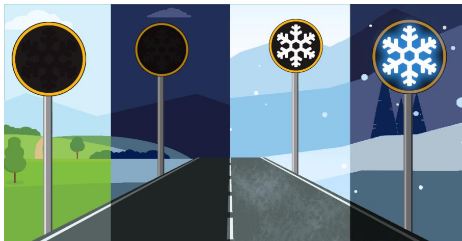
Figure 5.1 Illustration showing the application of the thermoresponsive icy road sign. In temperatures above 0 °C (left two images), the sign is in the 'OFF' state. When temperatures decrease below 0 °C (right two images) a white snowflake symbol appears, warning of the potential for icy surfaces. At night the sign is enhanced by temperature responsive fluorescence that only occurs below 0 °C.
