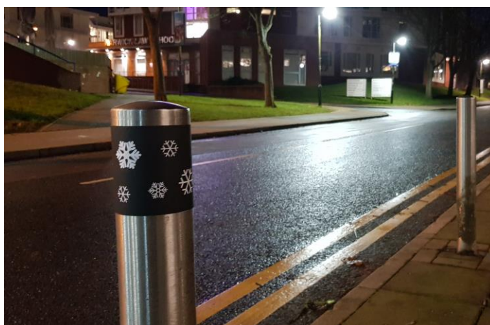
Figure 6.1 Full scale paper mock-up of thermoresponsive icy road sign.
