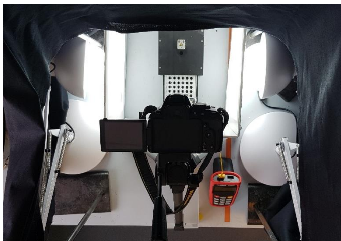
Figure 5.31 Photograph of multi-well photographic plate reader from above. A DSLR camera is positioned directly above the multi-well plate and two lamps are positioned on either side. During the measurement the top of apparatus was covered with black cloth to minimise ambient light.
