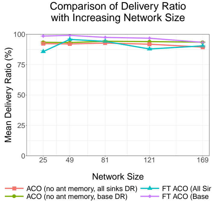
Figure 5.3: Comparing original ACO protocol with Fault Tolerant variant
