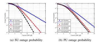
Fig. 2: OP as a function of transmitting SNR for SU and PU under different cognitive users M
