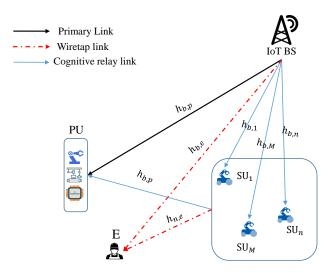
Fig. 1: Coexistence of a primary network and a cognitive multiply relay network. One primary user and M secondary users (SU) and a eavesdropper.
