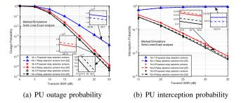
Fig. 7: OP and IP as a function of transmitting SNR for PU under two relay selection schemes
