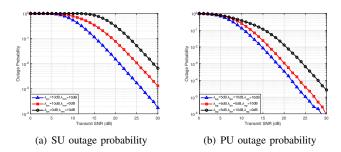
Fig. 3: OP as a function of transmitting SNR for SU and PU under different link conditions
