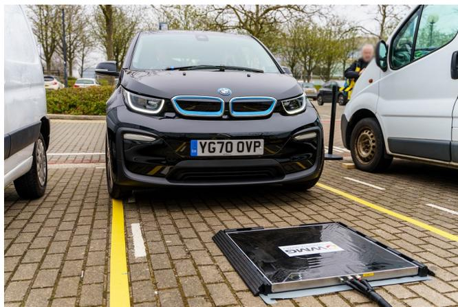
Fig. 13. Public mobile demonstration showing vehicle approaching wireless
