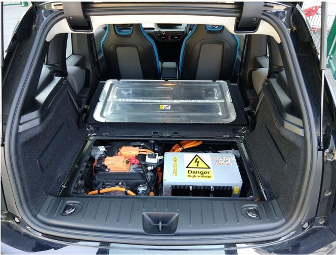
Fig. 9. Vehicle with fitted electronics box in the process of finalising the electrical and comms systems integration.
