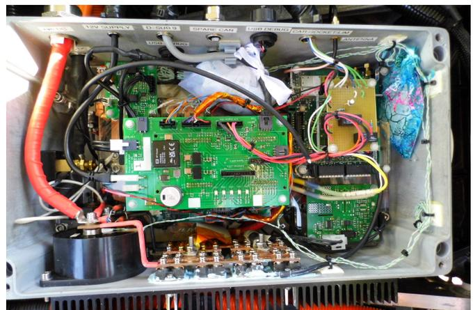
Fig. 7. Vehicle box internal architecture during construction, showing the layer approach and side-mounted rectifier.
