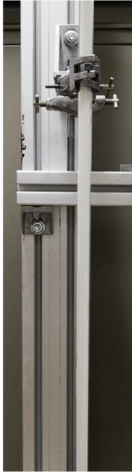
Figure 2. Gravity-driven granular flow through a pipe using particles with diameter between 100 and 200 \mu\text{m} and pipe with diameter 1.1 cm.
