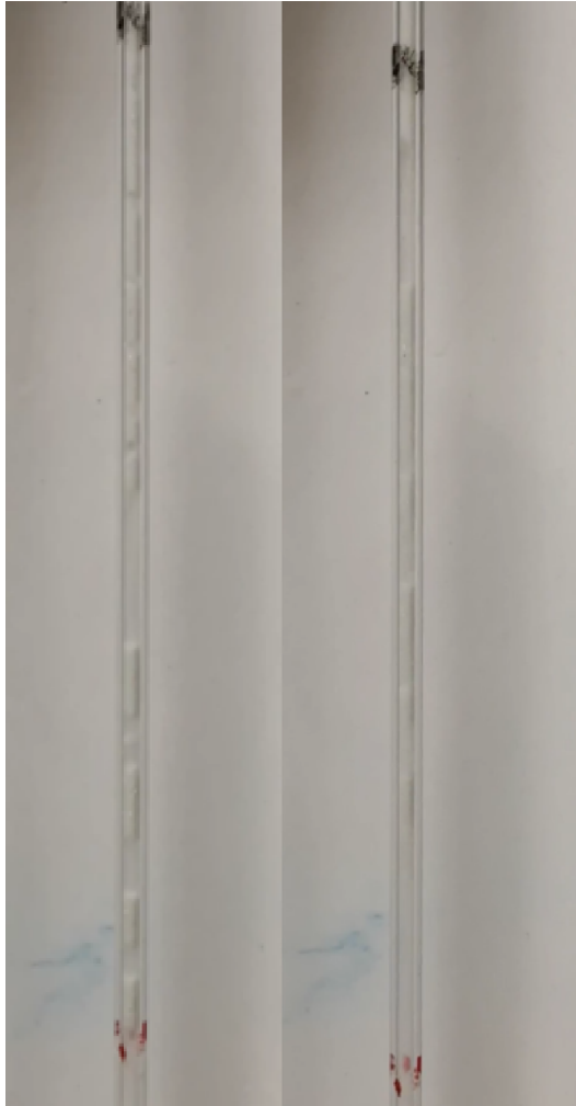
Figure 4. Almost stationary structure of density waves over a time period of 1.2 s.
