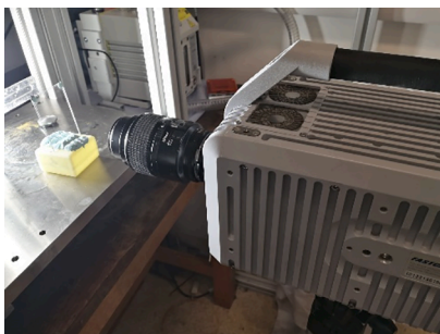
Fig. 2. Experimental set-up showing camera and pair of glass slides.
