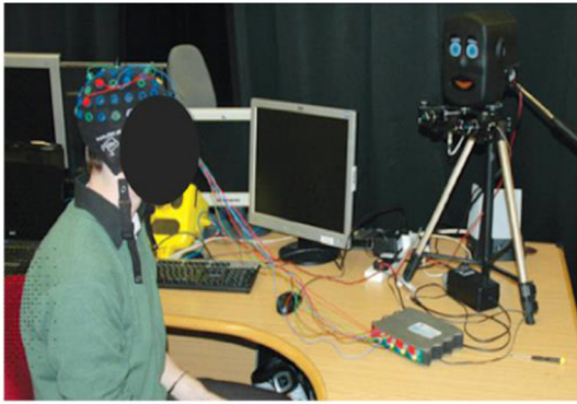
Fig. 3. EEG experiment setup with the participant seated in front of hybrid-face robot and monitor.
