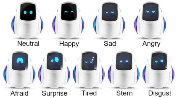
Fig. 6. Miko I social robot with a curved display resembling a 3-D structure of a face showing different emotions.
