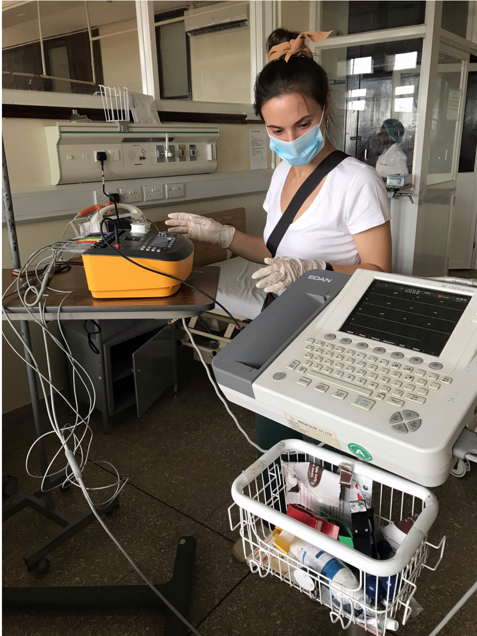
Figure 3.9: Electrical safety measurements
