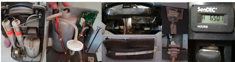
Figure 2.15: a, b Oxygen concentrator and its components; c, d details of dust and filters; e display with the number of hours that the device had been working [1].
