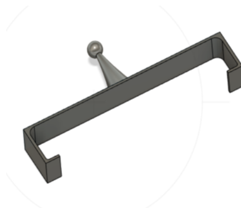
Figure 4.14: Smartphone add-on for vibration testing.
