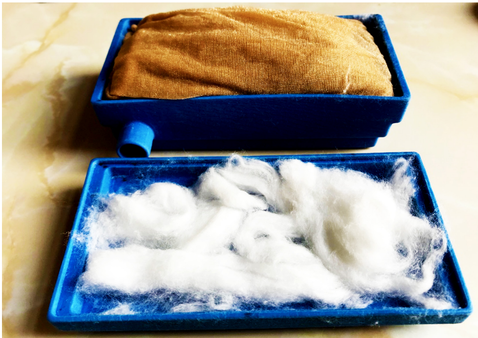
Figure 4.40: The 3D printed filter with the filtering material inside.
