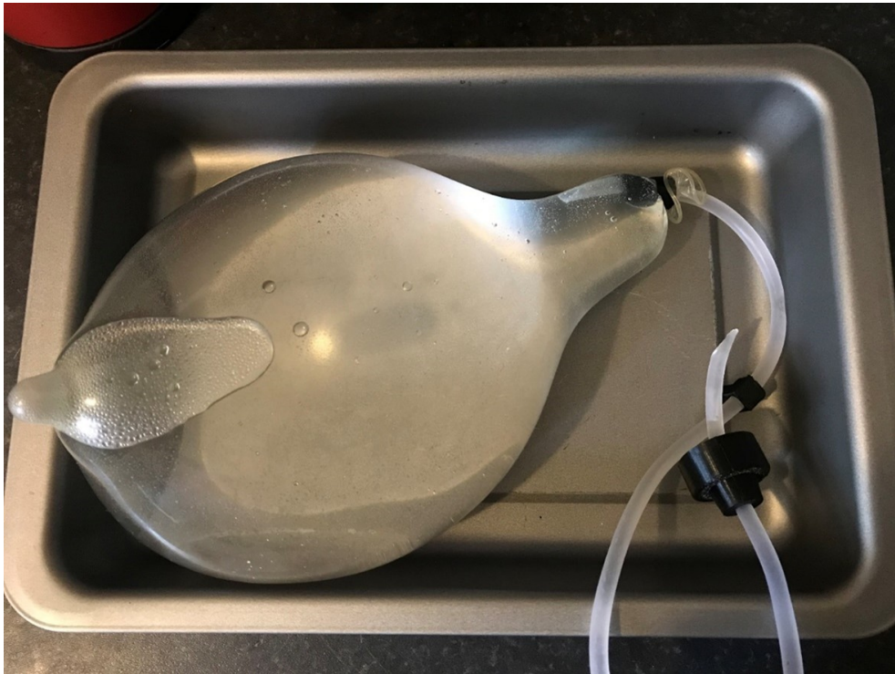
Figure 4.19: The setup of the open-air experiments: the condom filled with water and the flow-stopper that prevents the water from flowing back through the tube.
