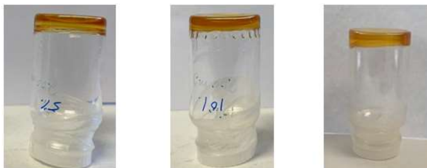
Fig 6. Pictures of the poly(DMA-MTM) 5% (left), poly(DMA-MTM) 10% (middle), and poly(DMA-MTM) 20% (right) gels before (top) and after (bottom) 48 hours of UV irradiation (365 nm, 15 mW cm -2 ) in DMF.
