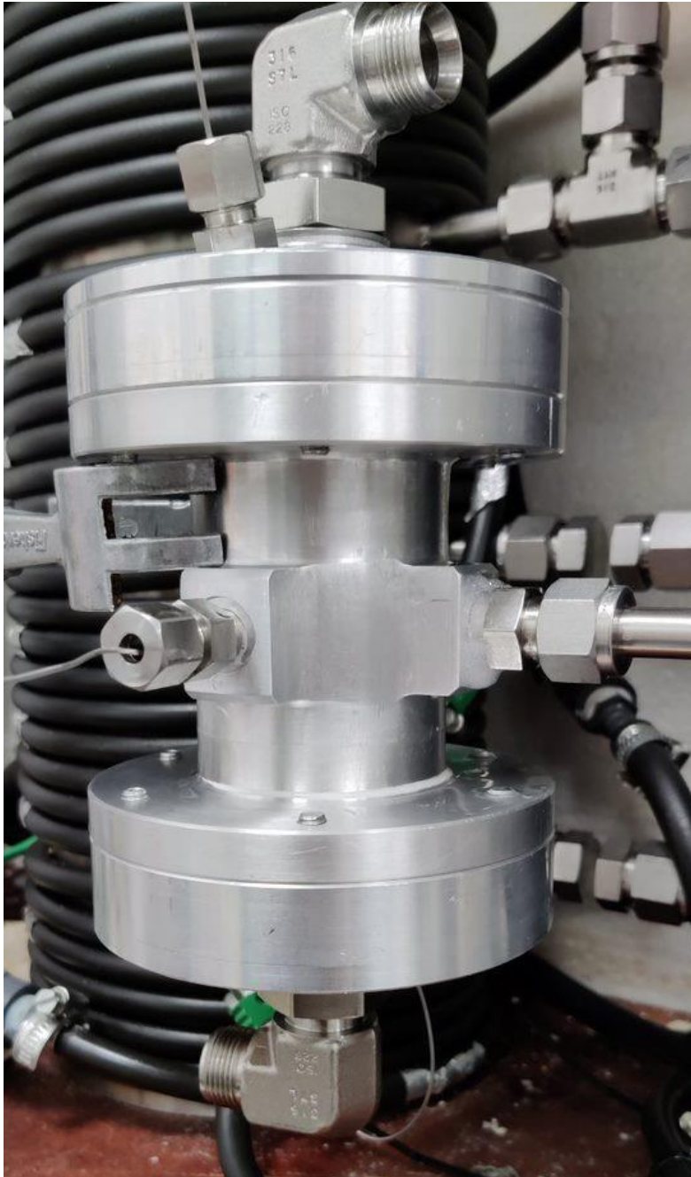
Figure 15 Shell side reactor. The main shell is manufactured from a single piece of aluminium machined down to include bosses to mount TC fittings and a BSP fitting to connect to expansion vessels. The two flanges also made from the same piece of aluminium, the top and bottom are tapped with BSP Swagelok elbow connection and gasket seal. The end of the shell is sealed with large silicone O rings and the 1/2" central tube is sealed with two silicone O rings.
