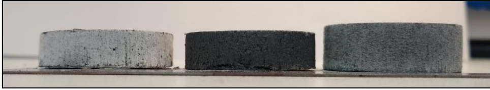
Figure 24 Picture to illustrate the difference in swelling of samples once used. Left to right: a sample dosed with barium chloride with limited swelling; ENG without salt; and a manganese chloride sample that has increased slightly in outer diameter and height.
