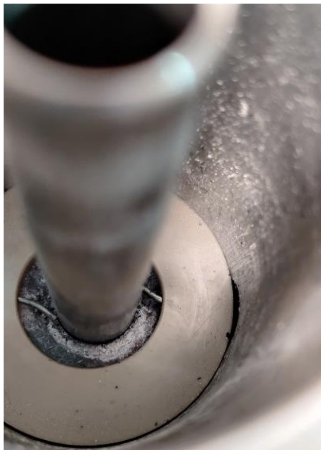
Figure 13 Grounded thermocouple contact with central pipe; a sample can be seen underneath.
