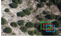
Fig.4. Illustration of the CIoU Loss. Key: Green box denotes ground truth T, blue box denotes the overlapping ground truth B, and red box denotes prediction P.
